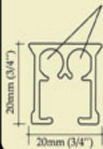
A two-channel rail system to prevent tangling of rope and provide a trouble-free mechanism
